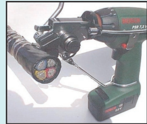
Metal tie installation tool
